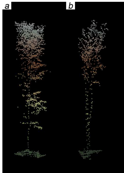
Figure 2: (a) 3D point cloud sample of a live tree, (b) 3D point cloud of a standing dead tree. Differences in vertical point distribution and point density are clearly visible.
